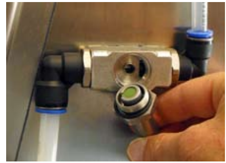
Fig. 8. Valve Stem removed. Clean the rubber-tipped end and inside valve black as needed.
