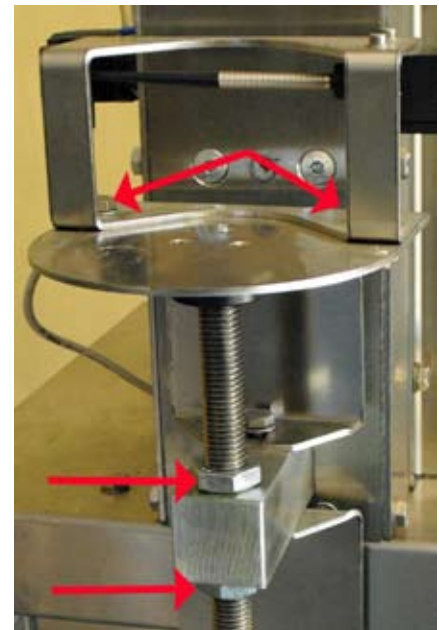
Fig. 2. Raise or lower bottle stand. Adjust Back Support to match Bottle Diameter.
