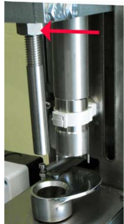
Fig. 4. Adjust Cork Pushing Pin to change depth of cork in bottle. ONLY MAKE THIS ADJUSTMENT AFTER BOTTLE HEIGHT ADJUSTMENT.
